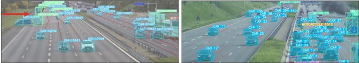
Figure 9 Visualization of the TUM Traffic Accident dataset with 3D box annotations, track IDs and trajectories.
